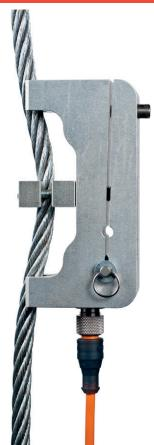
Working principle: The deviation of the cable caused by the intervention of the sensor causes a tangential force that is proportional to the force exerted on the traction cable. In the event of an overload, a microswitch integrated in the sensor is pressed and stops the electric wire rope hoist.
